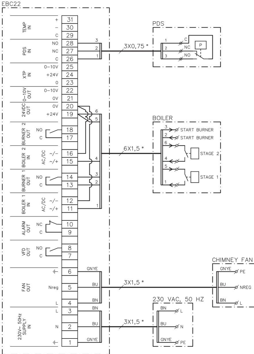
This example shows which inputs/outputs on the EBC22 need to be connected to a 2-stage boiler:
