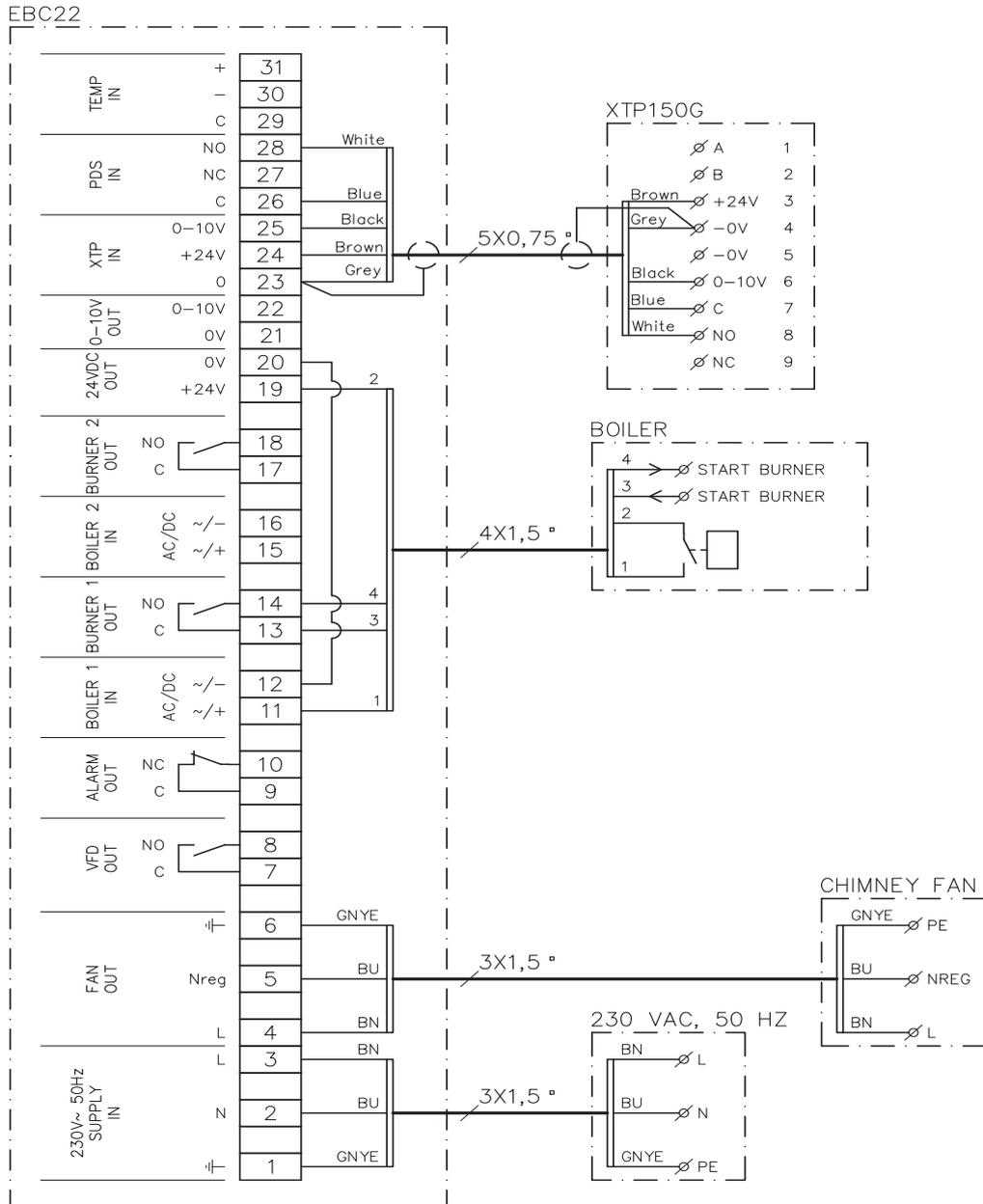
This example shows how to connect a potential free contact to the EBC22 to start/stop the fan
