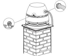
To avoid rainwater from entering the chimney 6 fan the slots and holes must be sealed with heat resistant and fireproof silicone.
