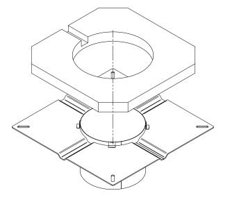
Fixate the flange to the chimney fan with the use of the vibration dampers supplied with the flange. The fan assembly can now be fitted onto the steel 5
