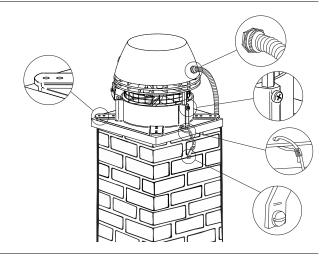
To avoid rainwater from entering the chimney 8 fan the slots and holes must be sealed with heat resistant and fireproof silicone.
