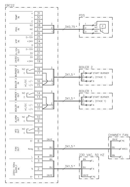
This example shows which inputs/outputs on the EBC22 need to be connected to 2 x 1-stage boilers. The boiler output for stage 1 is a voltage signal.
