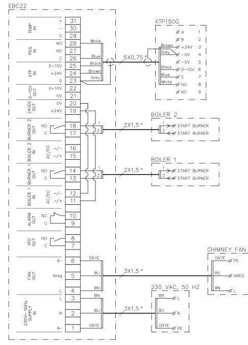
This example shows how to connect the EBC22 if you require continuous operation of the chimney fan from one or two boilers:
