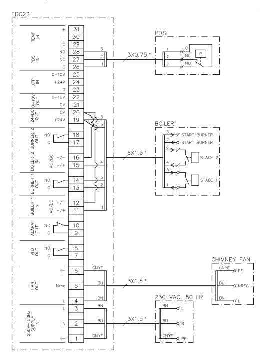
This example shows which inputs/outputs on the EBC22 need to be connected to a 2-stage boiler: The boiler outputs for stages 1 & 2 are two potential free contact sets.
