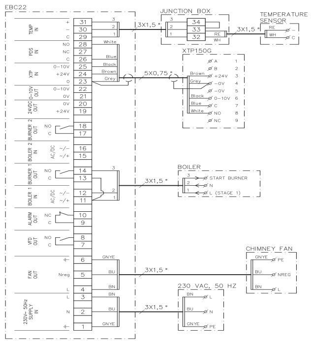
Example showing how a fan start/stop temperature sensor is connected to the EBC22.
