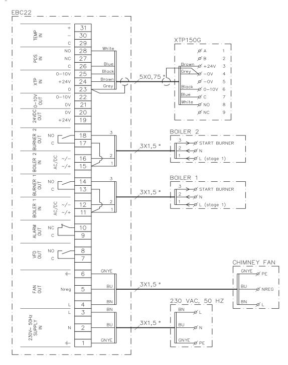
This example shows how to connect a voltage signal (10–230V AC/DC) for the EBC22 to start/stop the fan from one or two independent boilers:
