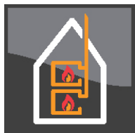
Decentralized multiple fireplaces connected to same chimney
