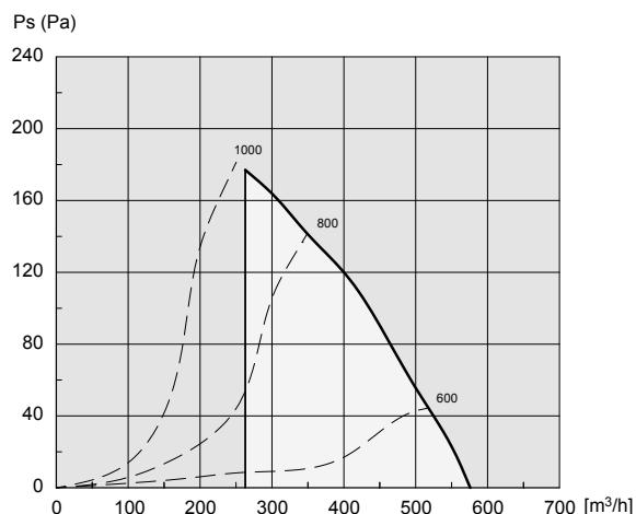
**PLEASE NOTE:** The capacity diagrams are measured with a flue gas temperature of 20 °C. The fan's capacity changes with the temperature of the flue gases. The correction of the capacity can be calculated using the following equation:
