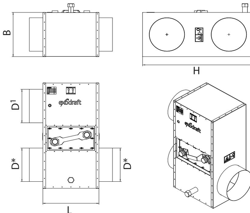
D\* = Muffenkupplung; D<sup>1</sup> = Spitzrohrende
