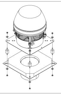
The fan assembly can now be fitted onto the steel chimney.
