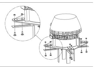
Adjust the distance between the location brackets to fit the inside diameter of the chimney, and then tighten the nuts. Note that there should be a 2-4 mm gap between the brackets and the chimney so as to avoid transmitting vibrations from the fan to the chimney
