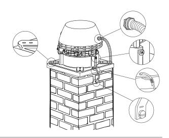
To avoid rainwater from entering the chimney 8 fan the slots and holes must be sealed with heat resistant and fireproof silicone.
