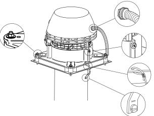
To avoid rainwater from entering the chimney 8 fan the slots and holes must be sealed with heat resistant and fireproof silicone.
