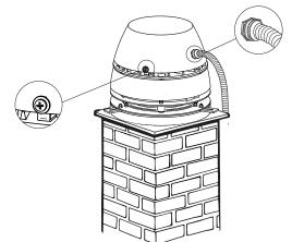
To avoid rainwater from entering the chimney fan the slots and holes must be sealed with heat resistant and fireproof silicone.
