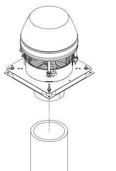
5 The fan assembly can now be fitted onto the steel chimney.
