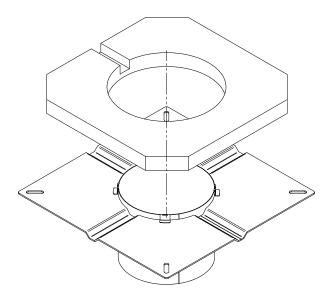
Fixate the flange to the chimney fan with the use of the vibration dampers supplied with the flange.
