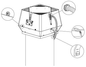
To avoid rainwater from entering the chimney fan the slots and holes must be sealed with heat resistant and fireproof silicone.
