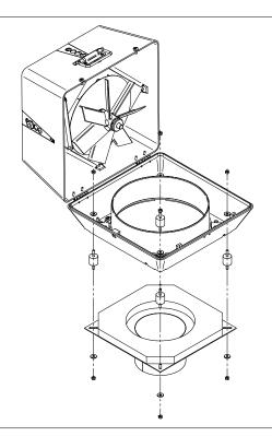
The fan assembly can now be fitted onto the steel chimney.
