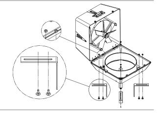
Adjust the distance between the location brackets to fit the inside diameter of the chimney, and then tighten the nuts.
