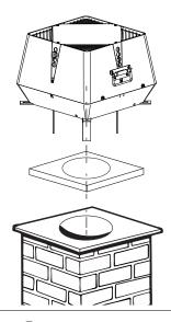
Use the safety wire to secure the fan to the chimney. Apply the supplied screw and rawlplug into the brick chimney. Then mount the wire through the designated hole in the base plate and into the wire lock.
