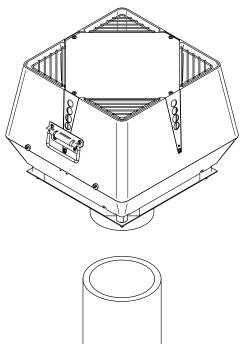
Use the safety wire to secure the fan to the chimney. Apply the supplied self-cutting screw in steel chimney. Then mount the wire through the designated hole in the base plate and into the wire lock.
