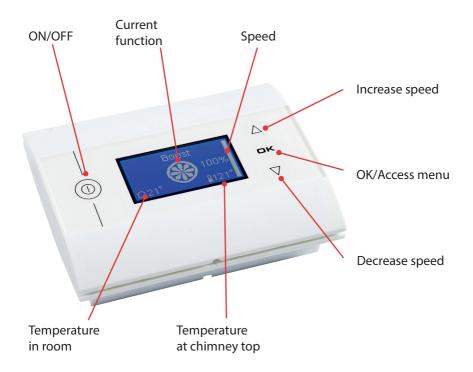
The display will turn on when pushing one of the buttons. After a short period it will automatically turn off the display.
